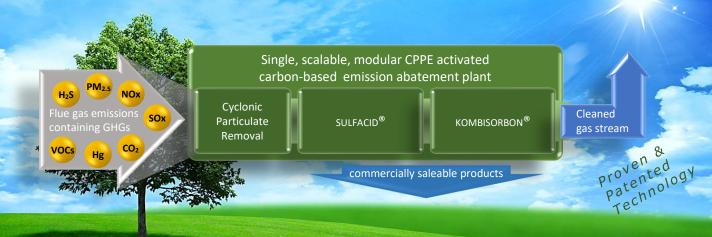
Reducing flue gas emissions today and into the future to meet tomorrow's regulations, while converting costly waste streams into commercial value-added products
