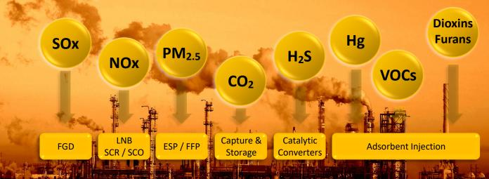
Multiple, separate technologies and plants for the partial abatement of flue gas emissions adding unnecessary capital overhead and life cycle operating costs
